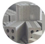
Bricks made from waste steel slag
