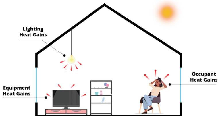
FIGURE 18: INTERNAL HEAT GAINS THROUGH OCCUPANTS, EQUIPMENT AND ARTIFICIAL LIGHTING
