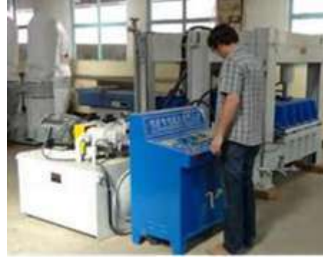
Press Machine (1000-2000 mm Length) Hot:10 15 Min Cold: 2 Hrs
