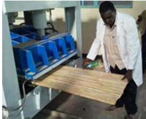
Press Machine (1000-2000 mm Length) Hot:10 15 Min Cold: 2 Hrs
