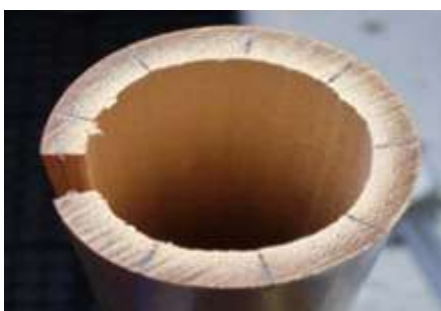
Step 4- Draw out thin bamboo sticks from the splits
