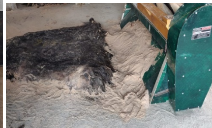
Desalting machine removes around 90 kgs of salt recovered from 100 hides
