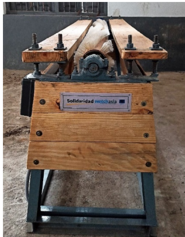
Desalting machine removes around 90 kgs of salt recovered from 100 hides
