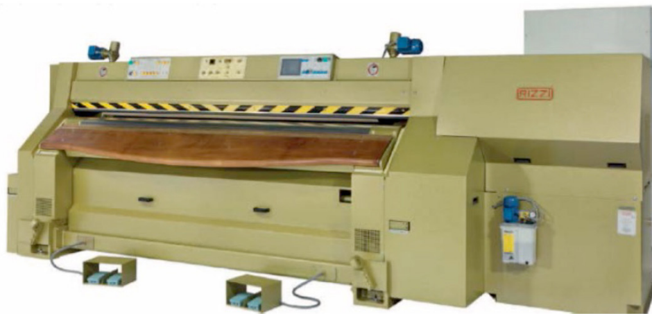
Figure 7: Shaving machine. Source: UNIDO
