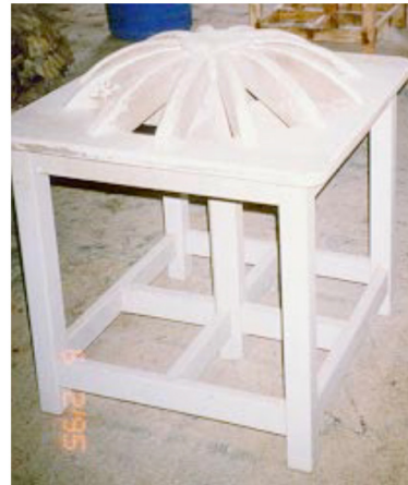
Figure 12: Dome-type DODECA wooden frame for manual desalting. Source: UNIDO
