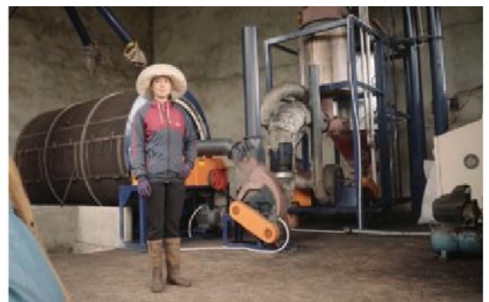
Pyrolysis system with drum dryer (left) manufactured by Viet Hien Co. and implemented at Binh Minh Cooperative
