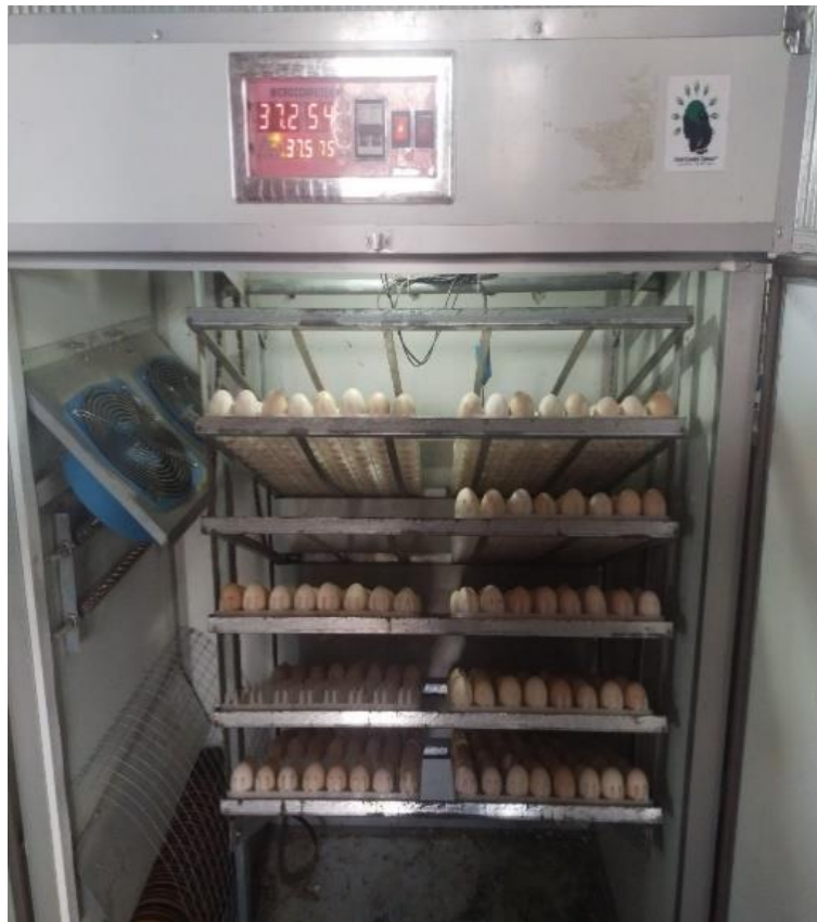
Figure 14: Solar Powered Egg Incubator
