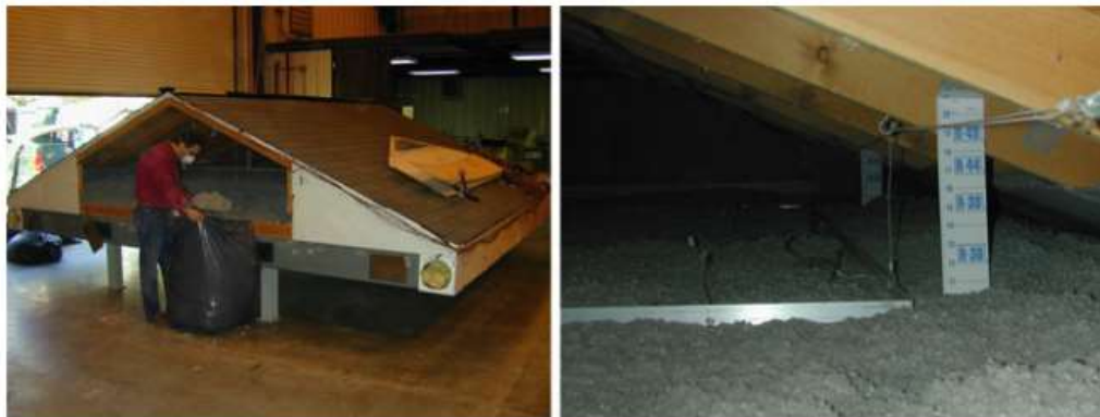
Figure 33: Experimental attic module containing microencapsulated PCM blended with cellulose insulation, ORNL, USA, testing facility. (Kośny, 2015, p.48)
