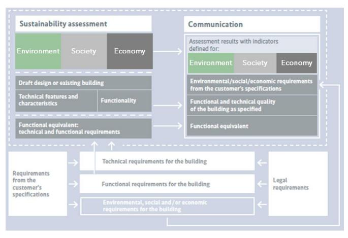
Figure 21: Flowchart of a sustainable building process Source: BMUB (2016)
