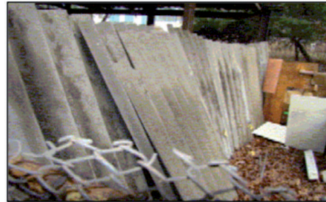
B. Storing old asbestos roof panels
