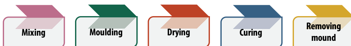
Figure 19 Overall process of reprocessing ash block
