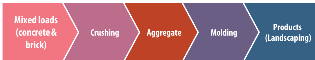
Figure 21 Overall flow of reprocessing masonry materials
