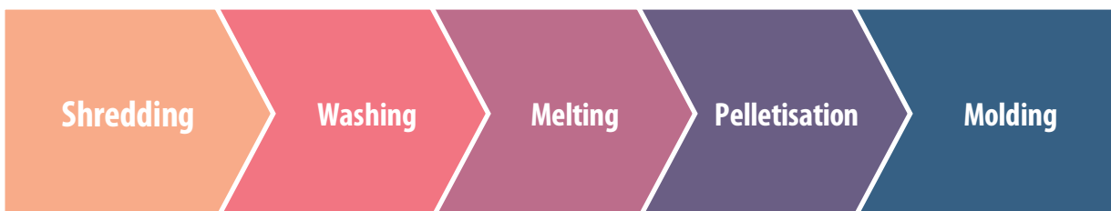
Figure 15 Overview of the reprocessing plastic flow
