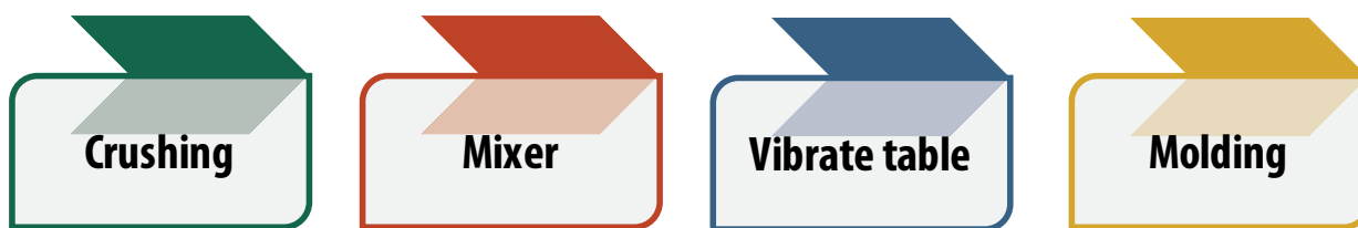
Figure 17 Overview of the flow of reprocessing glass
