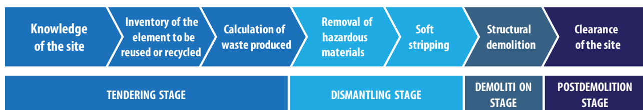
Figure 23 Overview of the Selective Demolition process
